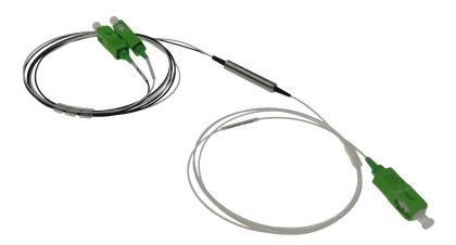
Gezhi Optical Fiber Filter WDM FTTX 1625nm is made by special optical components and advanced technology, it can deeply let 1600-1670nm wavelength pass but efficiently filter out 1250-1590nm wavelength. This product is mainly used in optical fiber on-line testing. It is ideal component of 1625/1650nm optical fiber filtering.
